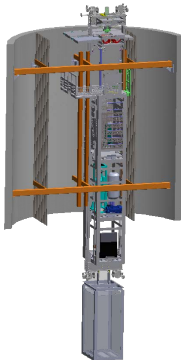
'Skip Style Work Platform'
